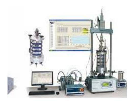
Triaxial testing of soils provides valuable soil strength and shear information for safe and effective design and construction of embankments and foundation systems. Build the optimum system for your application by selecting from Gilson's Load Frames by Karol-Warner, Master and Auxiliary Control Panels, quality Test Cells and test accessories.
